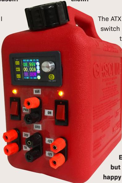
The ATX power supply I used does not have any way to switch off mains power, so I cut the hot line and included the switch. The other switch connects the green (power on) wire to ground.
